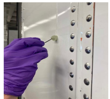
Figure 6. Applying Edge Sealer
