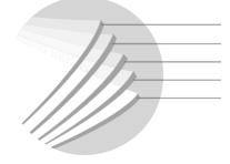
Cap Sheet – Polyester Clearcoat – Polyurethane Film – Polyurethane Adhesive - Acrylic PSA Liner - Polyester
